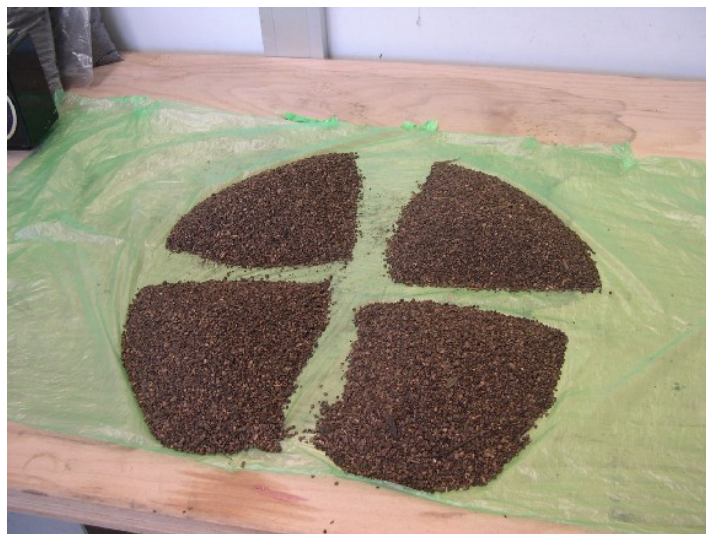
Figure 2. Photograph of the coning & quartering method using olive residues.
