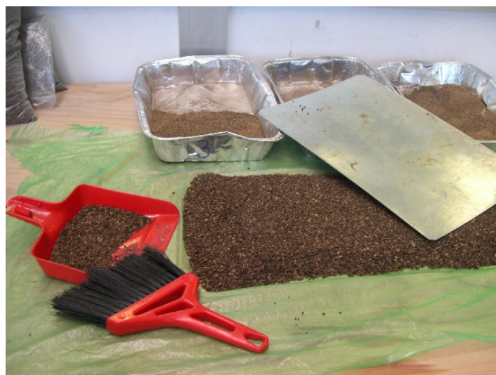
Figure 1. Photograph of the long pile method using olive residues.
