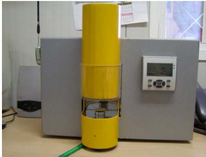
Figure 8: Compression machine to determine the pellet compression strength used by CIEMAT
