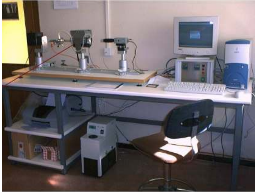
Figure 1: example of an apparatus according CEN/TS 15370-1 (source CIEMAT)
