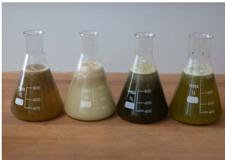
Figure 7: Water biomass blend left overnight in Erlenmeyer flasks
