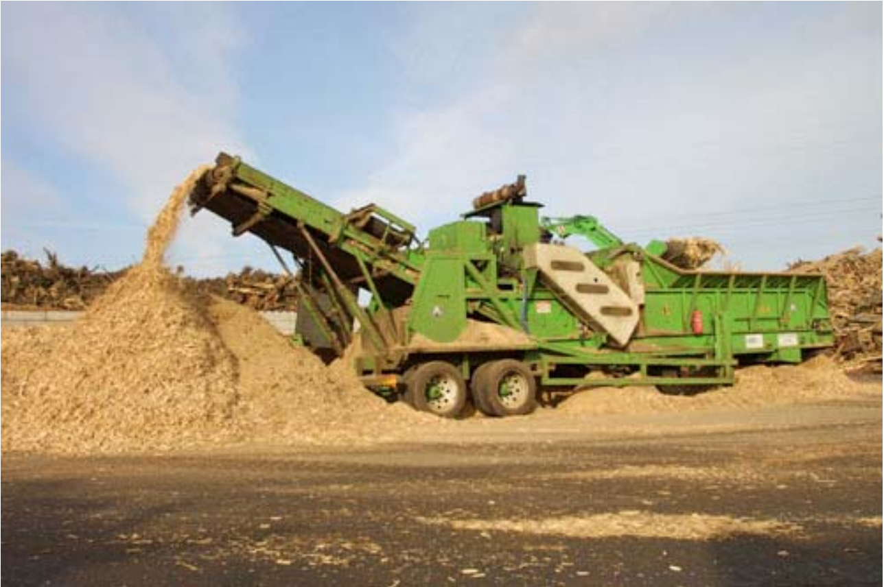
Figure 4 – Shredder to reduce the category B-wood size /1/
