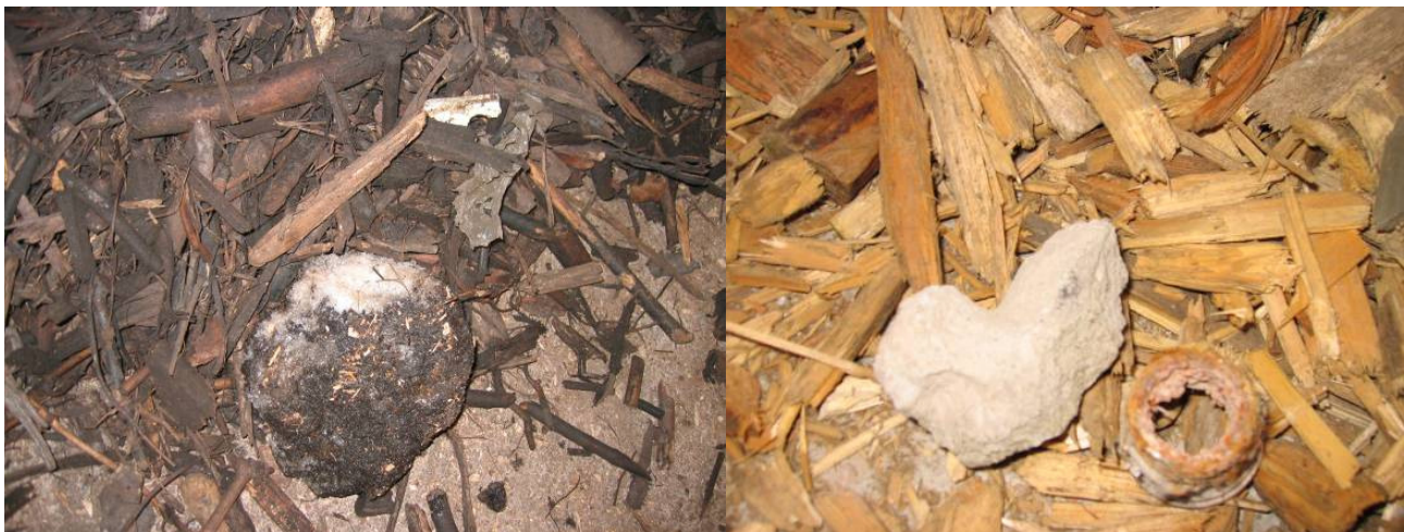
Illustration 9 and 10: impurities (stone and metal) in hog fuel [5]
