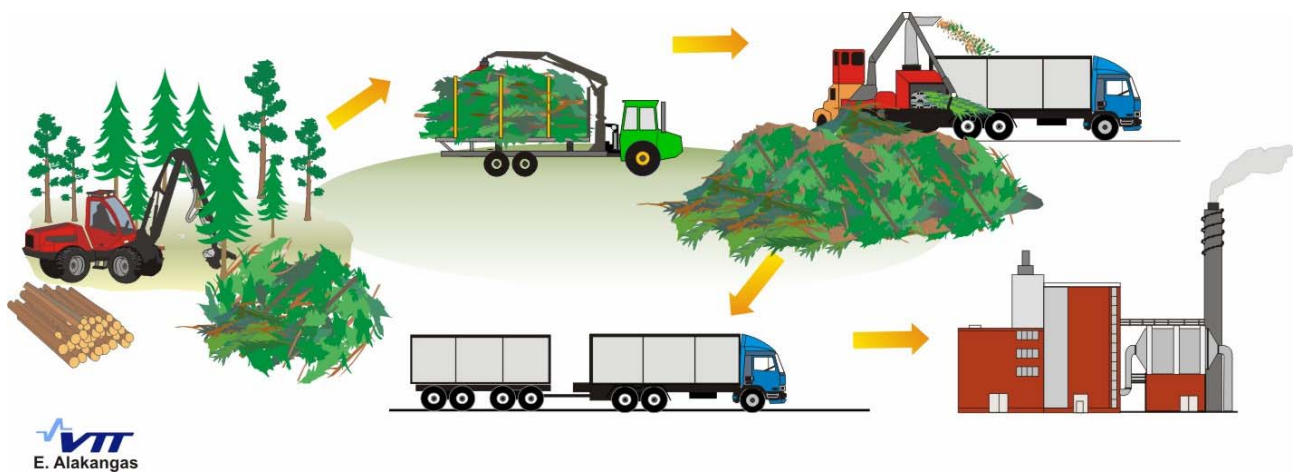
Figure 8. Logging residue supply chain – chipping at road-side most common production method, company C and E.
