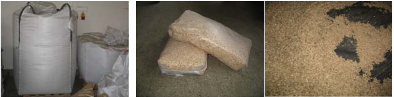
Figure 5. Wood pellets in big bags, 15 kg bags and in bulk form, company F.
