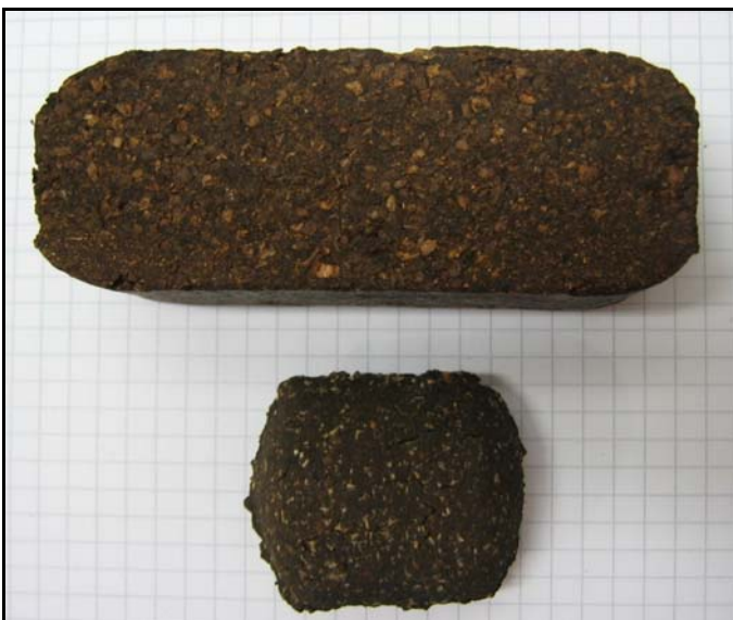
Figure 15. Exhausted olive cake in the traded form of briquettes supplied by case company A
