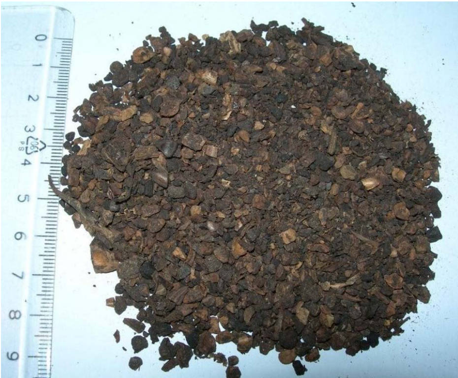
Figure 14. Exhausted olive cake in the traded form of grains supplied by case company A
