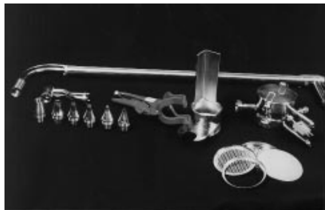
Probe unit ESS with zero-pressure nozzles, out-duct filter housing for 90 mm filters, cassettes and transport container, insulating cover, port hole adapter for RP 3"
