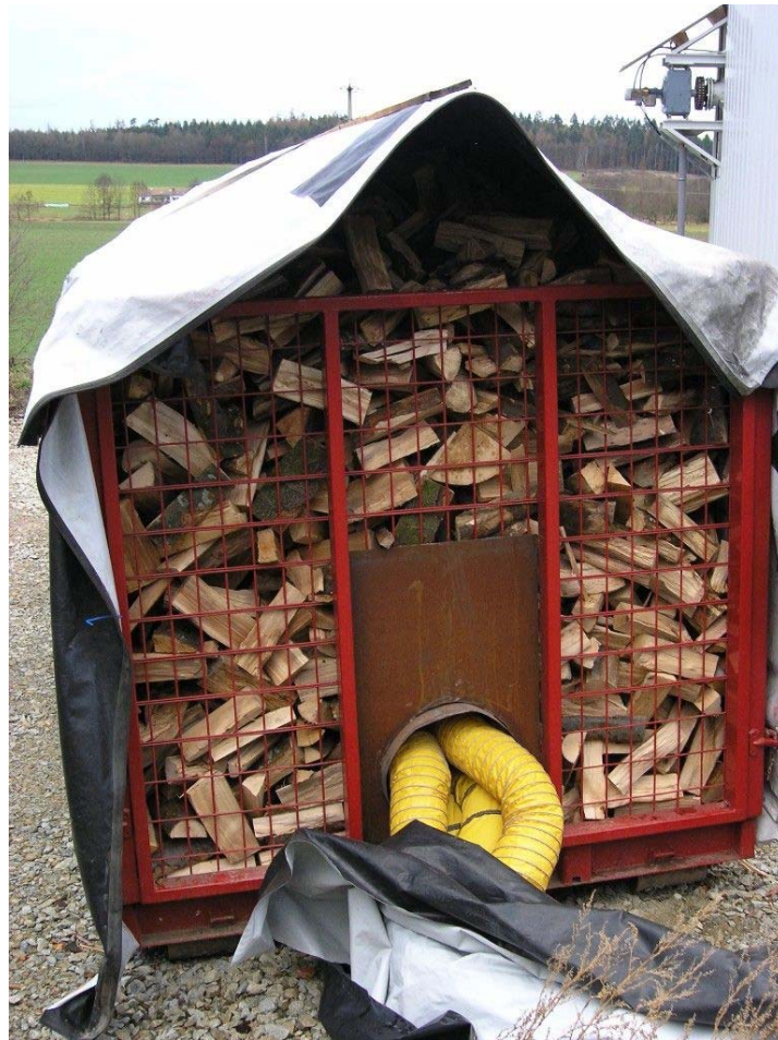
Figure 10: Simple container based appliance for artificial drying of wood logs using waste heat from biogas plants (Photo: TFZ)
