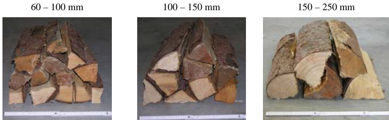
Figure 3: Hand sorted wood log diameters as used in the trials concerning the size effects
