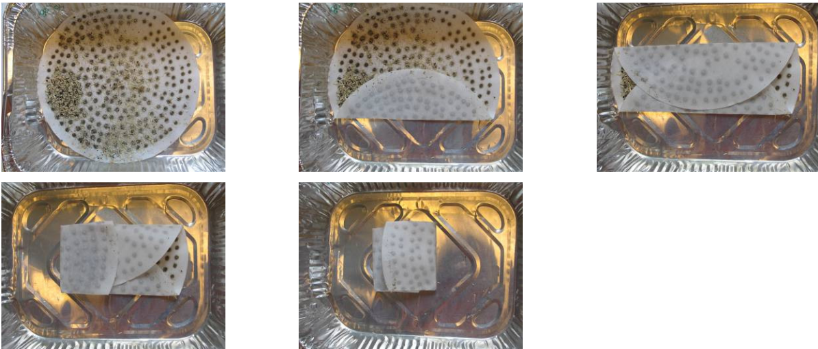
Figure 3: Procedure for folding the filter paper.
