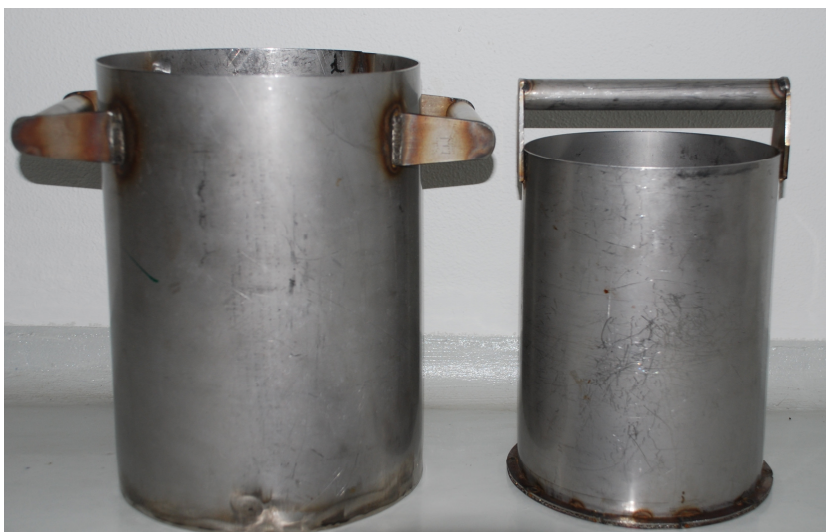
Figure 1: Inner (sample) and outer (flushing) container for detaching of mineral impurities by washing in deionised water.
