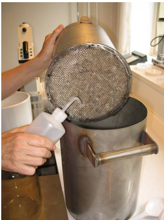
Figure 2: Gently tip the inner container and rinse any particles of the bottom of the inner container into the outer container.
