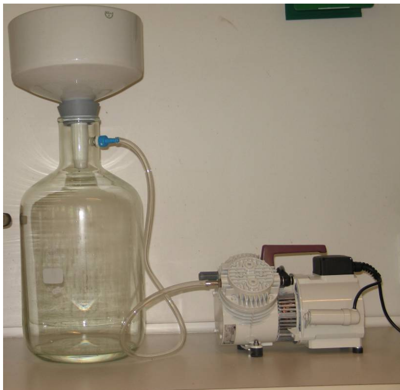
Figure 3: The vacuum pump is connected with the büchner flask and the rubber fitting; the büchner funnel is placed on the büchner flask.
