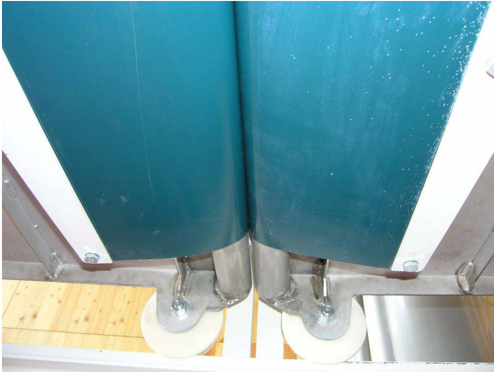
Figure 8: View from below on the closed opening slot (with movable floor and undercarriage)
