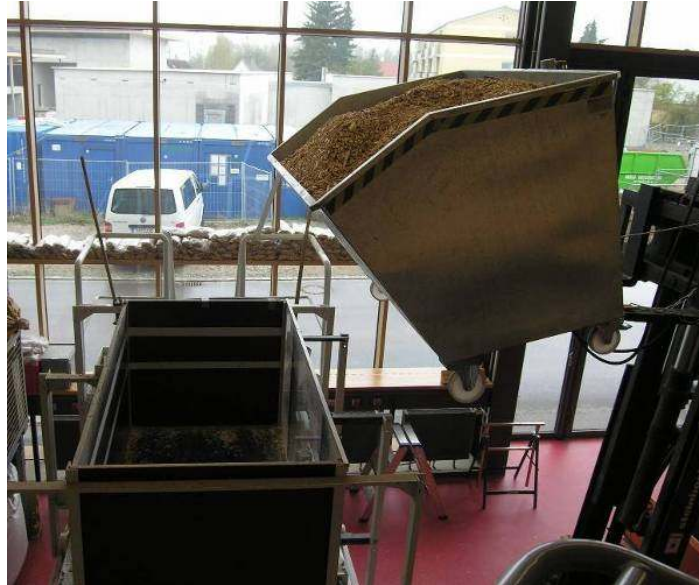
Figure 10: Filled tilting container mounted on a fork lifter before dropping the sample into the tester
