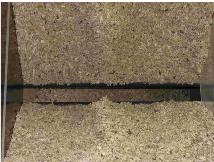
Figure 2: 100 % bridge collapse (view from top)
