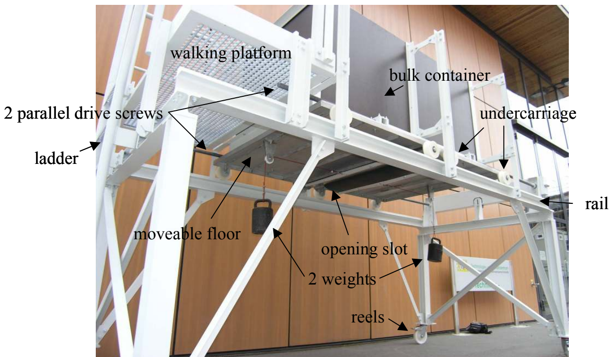
Figure 7: Description of the main constituents of the bridging tester
